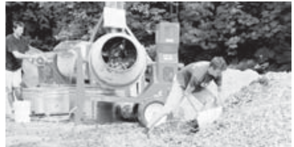
Cedar wood chips were delivered from a local mill, and an efficient production system was set up; mixing clay slip in a mortar mixer, then mixed with chips in a cement mixer.
