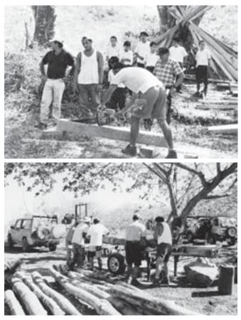
Top) Milling timbers with a chain saw at Finca la bella. Bottom) Milling melina logs in Tamarindo with a WoodMizer
